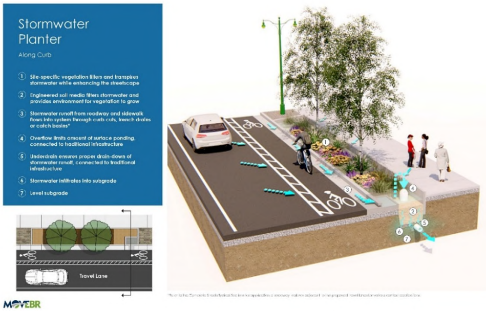
Figure 11-8: Stormwater Planter (along curb) Typology
