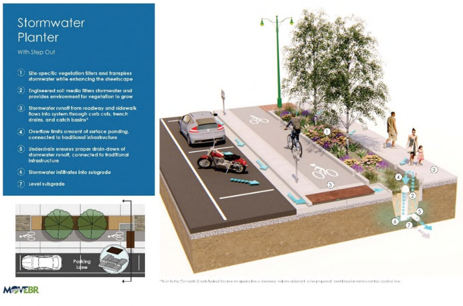
Figure 11-9: Stormwater Planter (with step out) Typology
